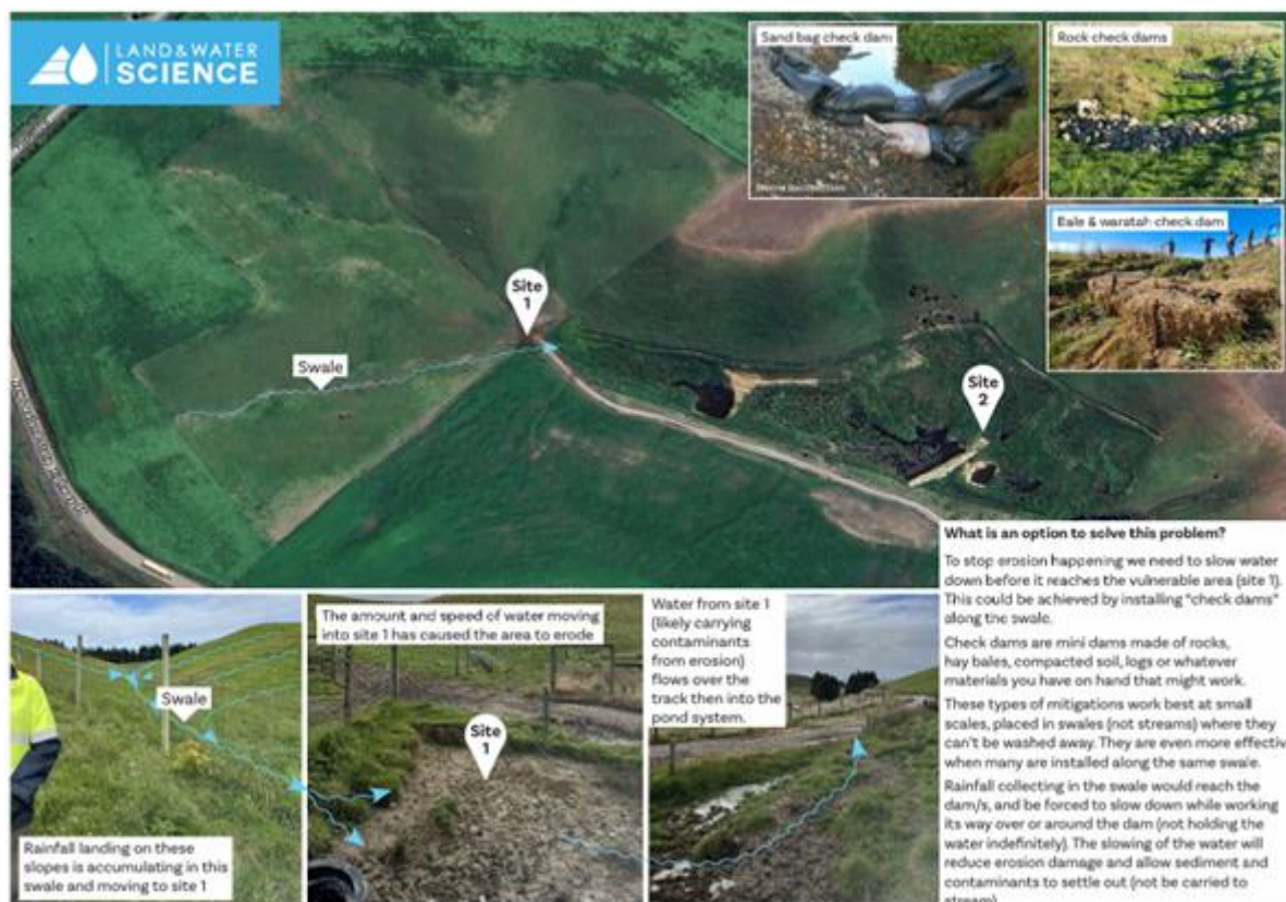
Figure 21. Example of a daisy chain of interventions along flowpaths. Note the use of a densely vegetated gully floor, wetlands, and multiple ponds to slow, trap, and treat runoff from areas of winter grazing at the head of the gully (courtesy Murray Ward, Gore Catchment Group).
